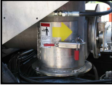
Auger access door with padlock in place
