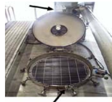
Locking tabs on hatch
