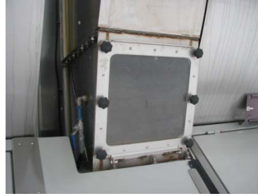
Surge hopper with tool-removable cover
