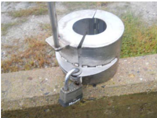
Lockable valve Locking Hood
